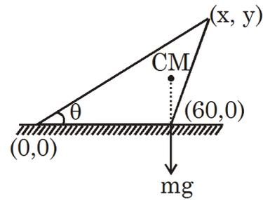
Just to prevent from toppling,  $mg$  must pass through toppling point.
