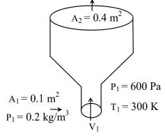
$$\begin{split} &\frac{dm}{dt} = \rho_1 A_1 v_1 = 0.8 \text{ kg/s} \\ &v_1 = \frac{0.8}{0.2 \times 0.1} = 40 \text{m/s} \\ &g = 10 \text{ m/s}^2 \end{split}$$
