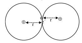
Hence potential energy will be calculated for 2 H atoms. (P.E. due to attraction of proton & electron)
