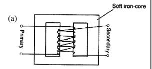
Working principle- Step-up transformer is made up of two or more coil wound on the iron core of the transformer. It works on the principle of magnetic induction between the coils. Whenever current in one coil changes an emf gets induced in the neighboring coil (Principle of mutual induction)
