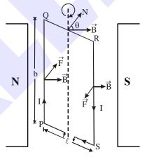
Let I be the current flowing through the coil PQRS,  $\ell$  and b are the sides of the coil PQRS.
