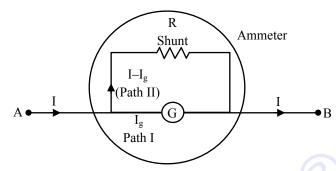
In parallel grouping of resistances, potential must be equal
