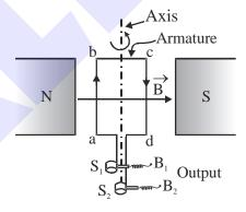
Working: When the armature coil rotates between magnetic poles with constant angular velocity  $(\omega)$  then the magnetic flux linked with the armature coil changes with time. The magnetic flux passing through coil is given by
