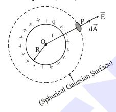
Using Gauss law, at a point P situated outside the sphere,
