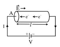
Where  $R = \frac{ml}{nAe^2\tau}$  is constant for particular conductor at a particular temperature and is called
