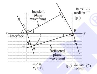
If velocity of light in denser medium is  $v_2$ , then distance travelled by wavelets in time t:  $AA' = v_2t$  Taking 'A' as centre and draw a spherical arc of radius  $AA' = v_2t$ . Now draw a tangential plane A'B' which touches the spherical arc at point 'A'. This tangential plane A'B' acts as a refracted plane wavefront.
