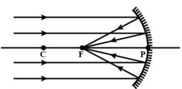
In a concave mirror, all the incident rays parallel to principal axis actually pass through the focus F after getting reflected from the concave mirror. Thus, concave mirror has a real principal focus.
