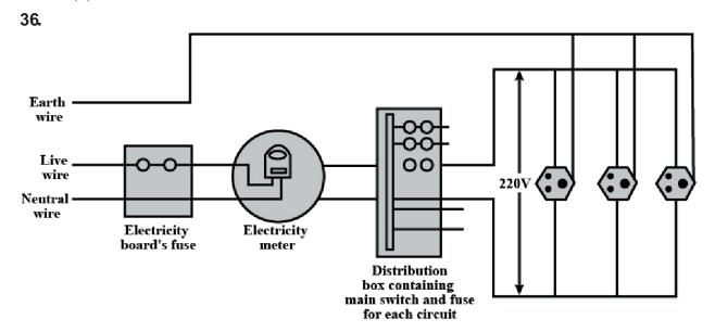
A fuse in a circuit prevents damage to the appliances and the circuit due to overloading. Otherwise, the appliances or the circuit may be damanged.
