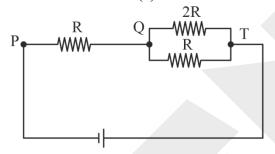
$$V_{PQ} = I^{1}R : V_{QT} = I^{1} \times \frac{2R}{3}$$
