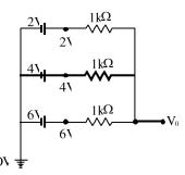
By nodal analysis  $\frac{V_0-2}{1k\Omega} + \frac{V_0-4}{1k\Omega} + \frac{V_0-6}{1k\Omega} = 0$
