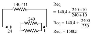
$\therefore \text{ Current in ammeter} = \frac{24}{150}$ = 160 mA
